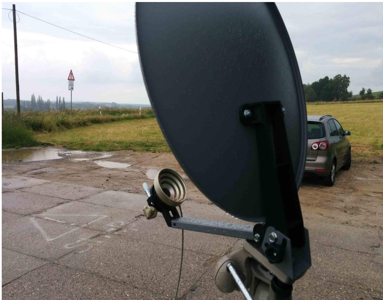
DH5YM-Station in JO61XA: 40cm camping dish used for 10GHz -the feed is the W1GHZ duoband feed
